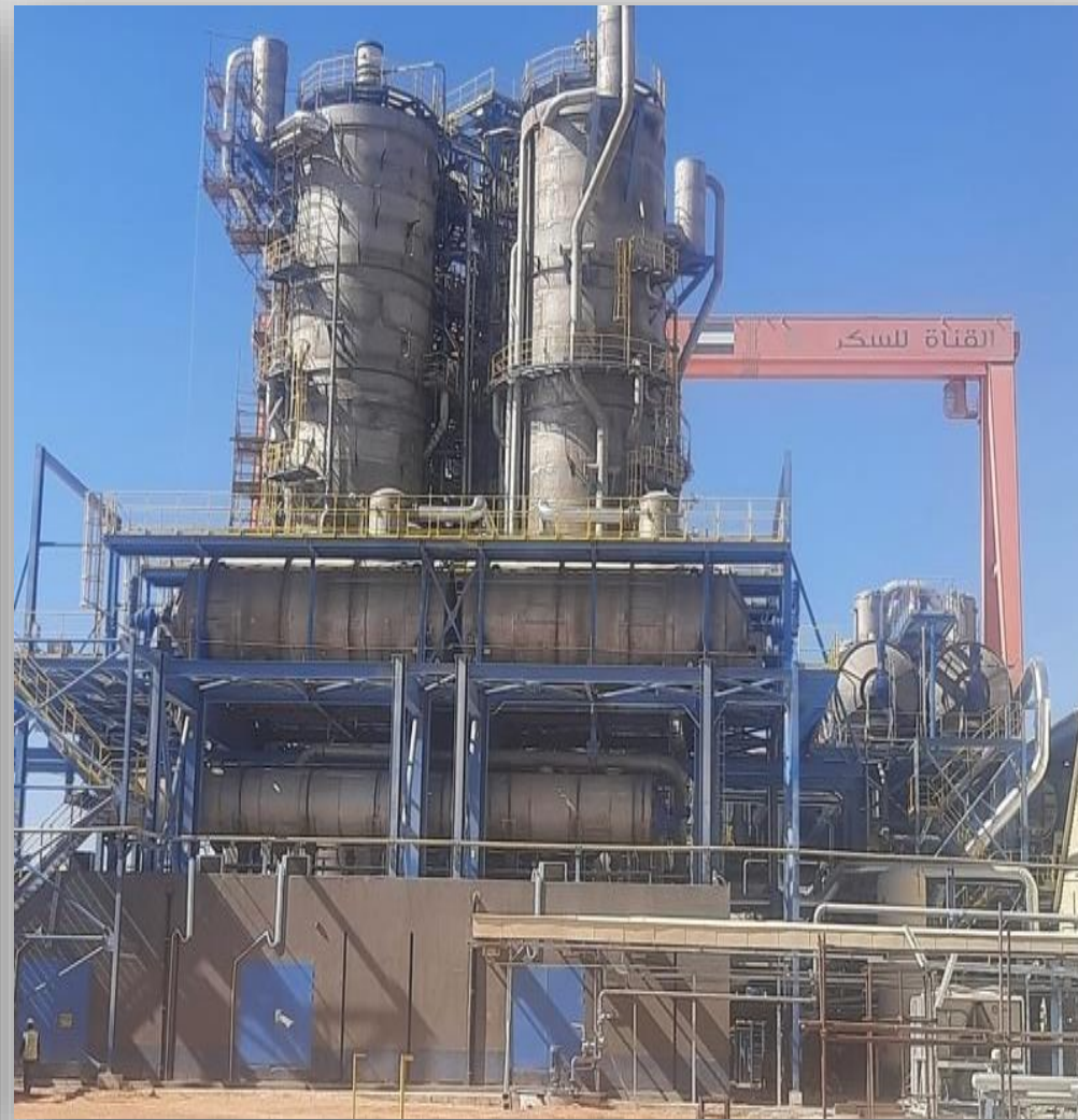
Centrifugal stations (CVC A,B & C) “Biggest in the world” Width 15m X Length 75m Height 15m
