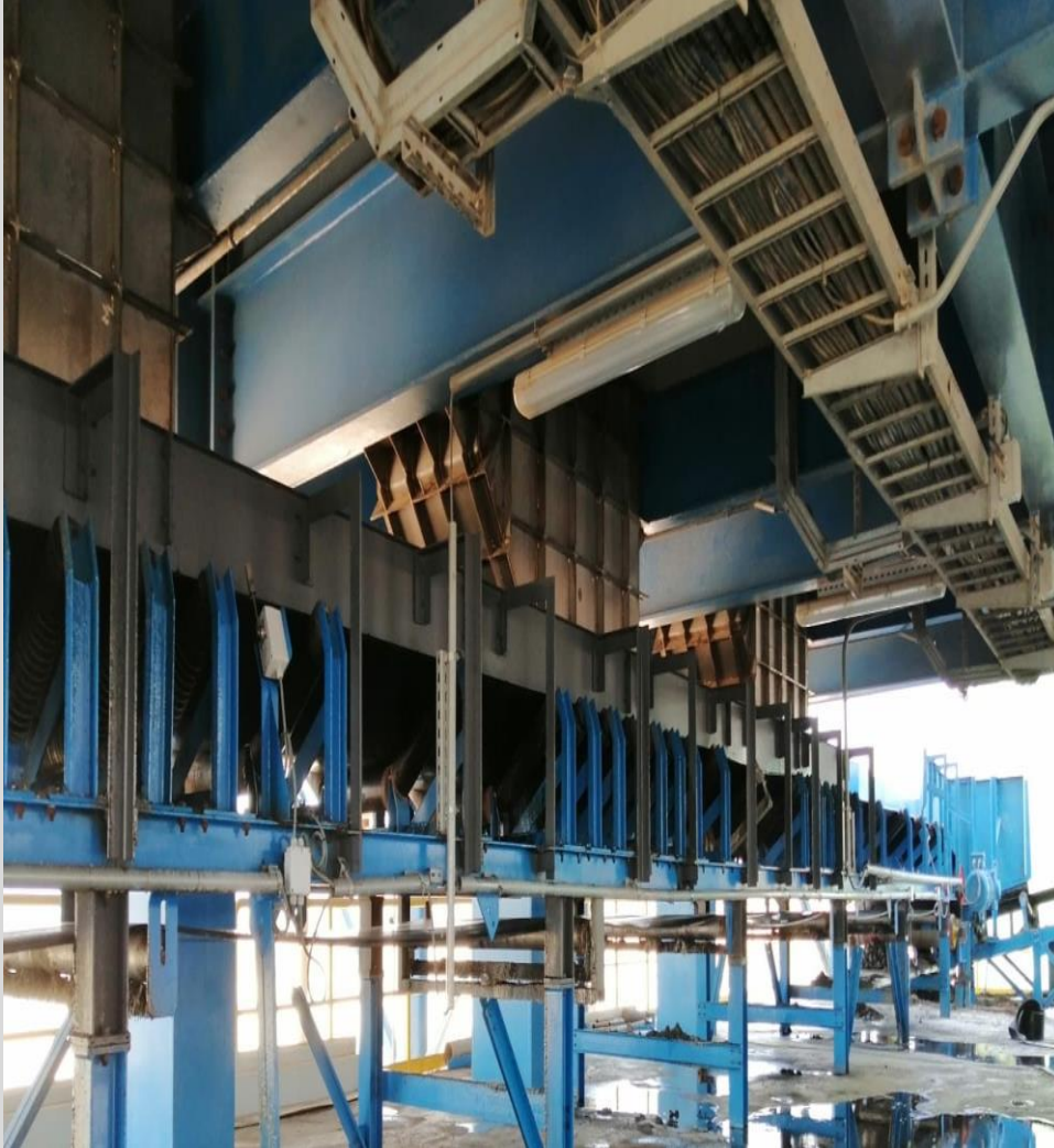
Dirty Beet Conveyors (Qty.2) Capacity 1,500 Ton / Hr.
